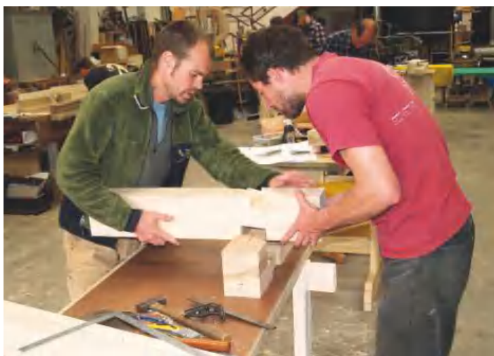
▲ Pic.15 Final fit – everything must be carefully aligned as the sections are large and the joints are tight
